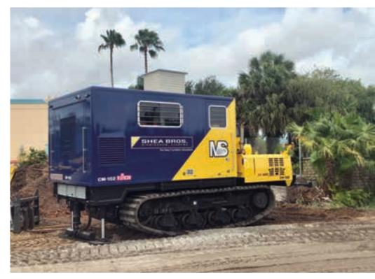
Cone penetration testing at a test area
